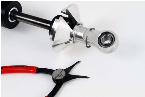
Figure 4 – Removing the Snap Ring
