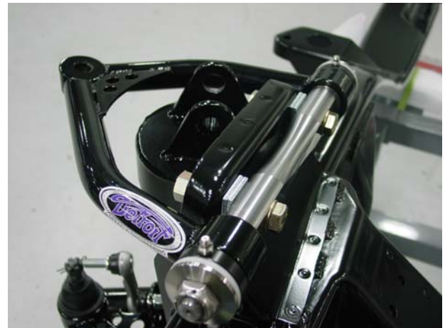
Figure 10b - Installed Upper Control Arm View
