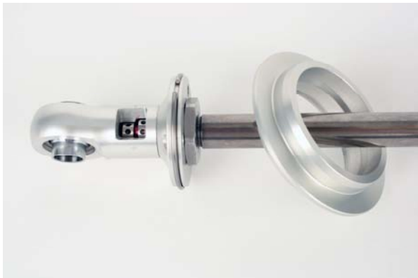
Figure 7 - Removing the Upper Spring Seat
