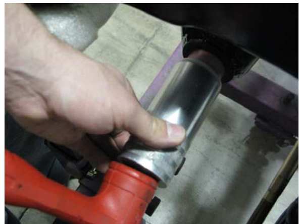
Figure 14 – Fully Installing the Bushings
