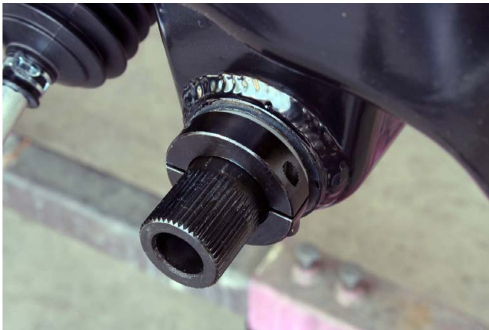
Figure 16 – Indexing the Clamp
