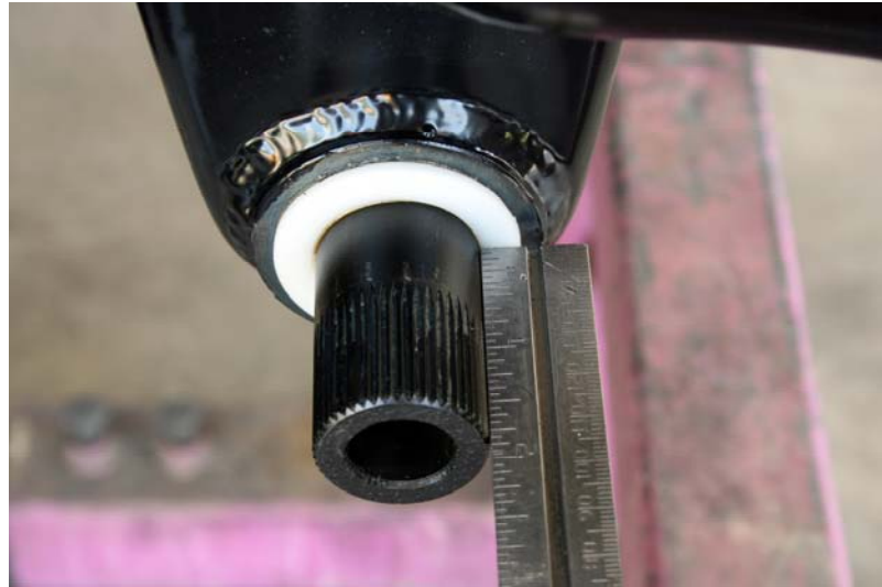
Figure 15 – Measuring the Anti-Roll Bar
