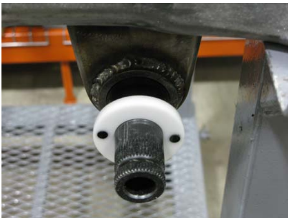
Figure 13 – Installing the Bushing & Anti-Roll Bar
