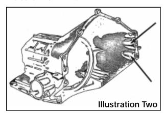
Note: Works only with small bolt pattern torque converters. If during installation your flexplate shield does not fit properly inside the transmission bellhousing you may need to modify the transmission case bellhousing. We have seen this condition with some of the
