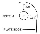
DO NOT TRIM LESS THAN .625 FROM ANY HOLE EDGE TO OUTSIDE OF PLATE!! N.H.R.A. Accepted Starter Hole
