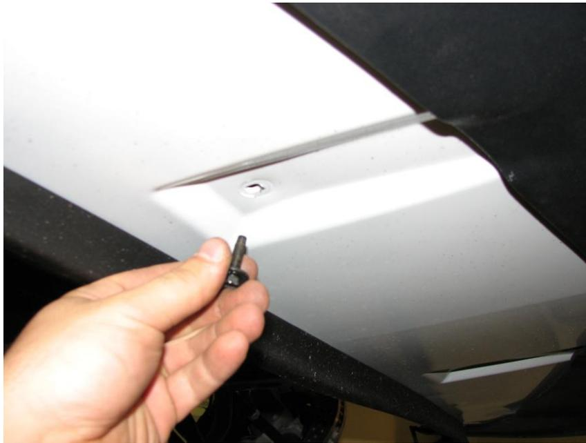
**Figure 5: Removal of 2 fascia support bolts**
