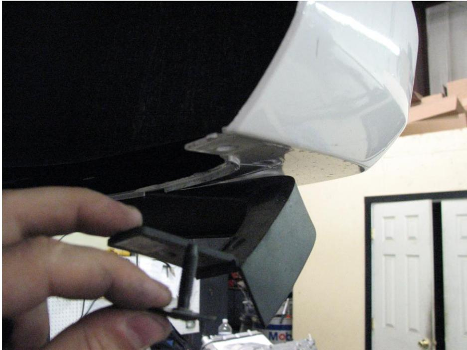
**Figure 1: Removal of 2 outermost fasteners**
