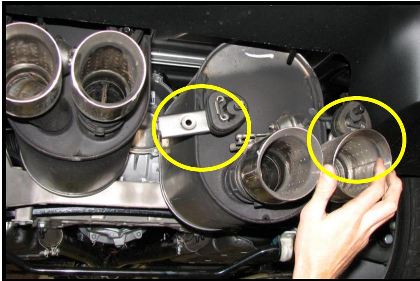
**Photo 2: Two of Four Muffler Hangers and Isolators**
