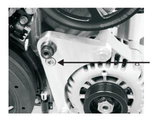
Install 10mm x 80mm SHCS through the bracket, through a 2.110" spacer and thread into the block.
