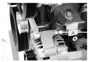
Install 10mm x 90mm hex bolt and washer through the bracket, through the alternator, then through a .250" spacer and last thread into the block.
