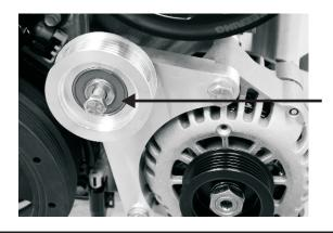
Install idler pulley with the 3/8" x 1 bolt, washer and lock washer. Make sure the steel black spacer is behind the idler pulley. Torque to 30-35 ft. lbs.
