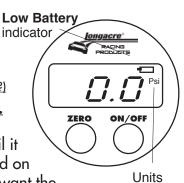
**TO CONVERT TO METRIC** turn unit on, then push and hold ZERO until it flashes. Release ZERO, then push again to change. Units are displayed on the right side. Options are: psi. BAR, & kPa. When you get what you want the gauge reverts to normal function in 3 seconds and stays until you change it again.
