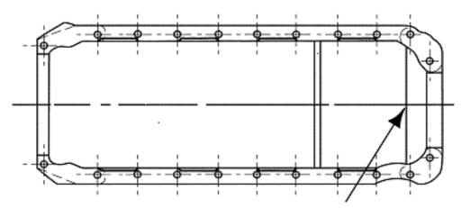
May have to be notched for clearance when pan is used with high volume pump.
