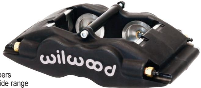
These new **FSLI4** and **FSLI4/ST** models use the latest innovation to the **Superlite** family of calipers. They have been redesigned with internal fluid ports that eliminate the external fluid cross-over tubes. The transfer tube has been replaced with two additional bleed screw assemblies which allow this group of right and left hand oriented differential piston bore calipers to be mounted in either a leading or trailing position.
