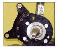
Photo 1 (Drum Spindle Mounting)
