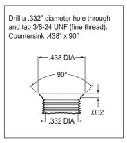
Figure 3. Drill and Tap Detail
