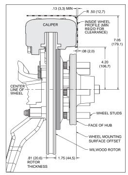
Figure 4. Wheel Clearance Diagram
