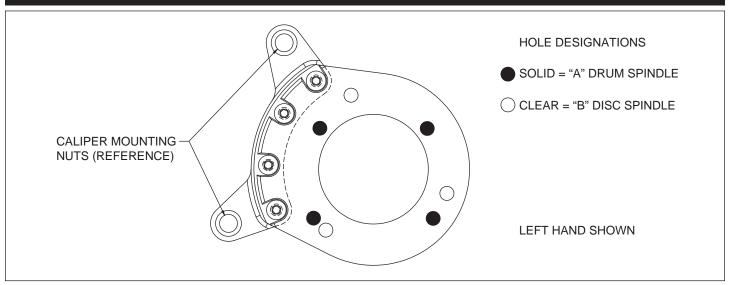
Figure 1. Wilwood Caliper Mounting Bracket
