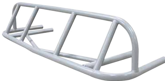
Kit shown assembled and must be welded
