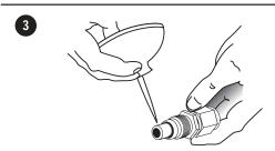
${\it 3.}$  Lubricate the inside of the hose, the cutter threads and the socket threads with Earl's assembly lube or engine oil. Place the nipple in a vise.
