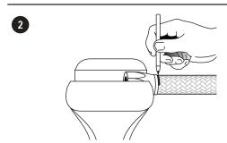
2. Place the socket in a vise and insert the end of the hose into the socket until the hose butts against the bottom of the threads provided for the cutter. Gently pull the hose back until there is a 171-6" to 178" gap between the end of the hose and the bottom of the threads —mark hose at bottom of socket with a felt pen so that you can detect any tendency of the hose to be pushed out as you complete the assembly.
